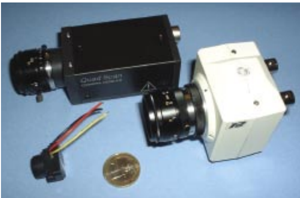
An active (LED illumination) or passive target is viewed by a camera. A specific software is used for the image grabbing and data processing.
