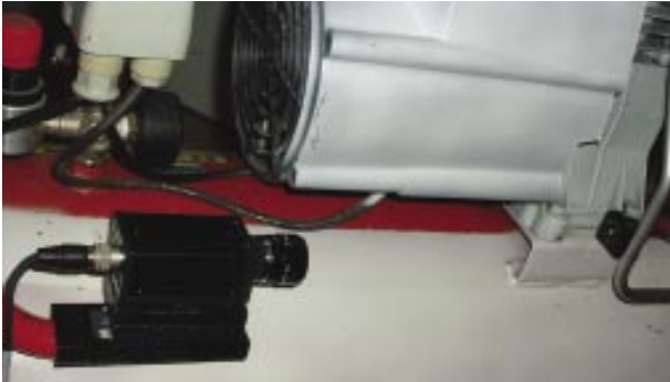
Measurement of engine movement of an air compressor.
