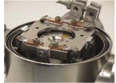
The sensor mounted in the cryogenic chamber (80 K).
