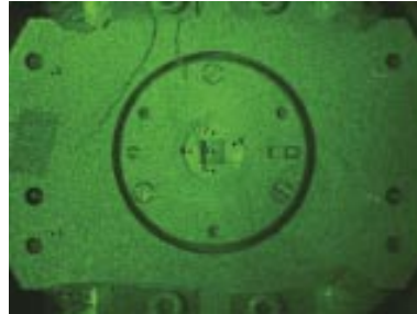
View of the sensor illuminated by a laser. The measurement has been done on eight points simultaneously
