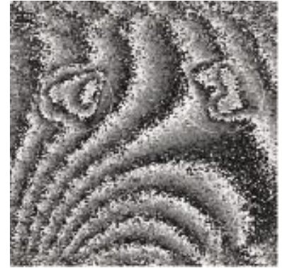
Artificial faults on an elastomer test specimen - SEP division of SNECMA
