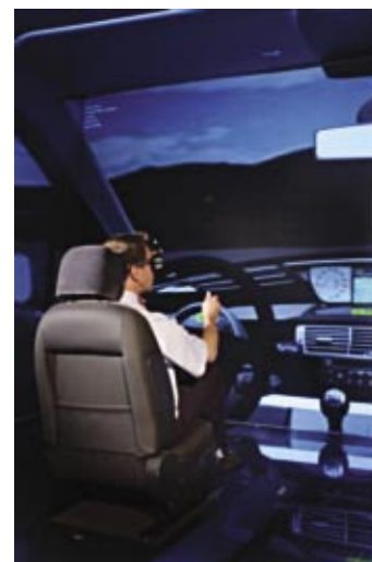
Ergonomics study of the interior of a vehicle - PSA
