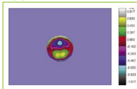
Difference between measured points and a perfect sphere (mm)
