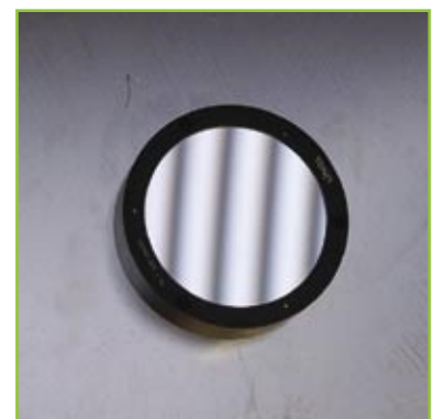
Curvature measurement of a concave mirror
