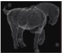
The cloud of point of the 3D digitised object. Several 3D views are merged to obtain the complete object.
