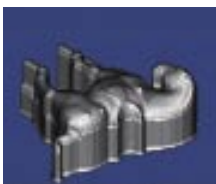
The post-processing of the clouds of points have been done by DELCAM using COPYCAD and POWER MILL software.
