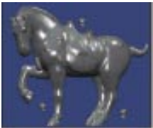
A triangulation is done that can be used for milling or rapid prototyping.
